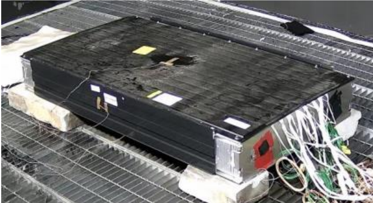
Figure 5 Tray tested to UL 9540A module level testing.
